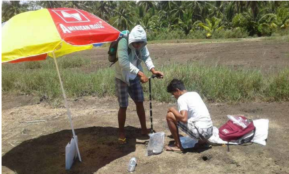
Figure 2.1 Auger Boring and Soil Sampling
