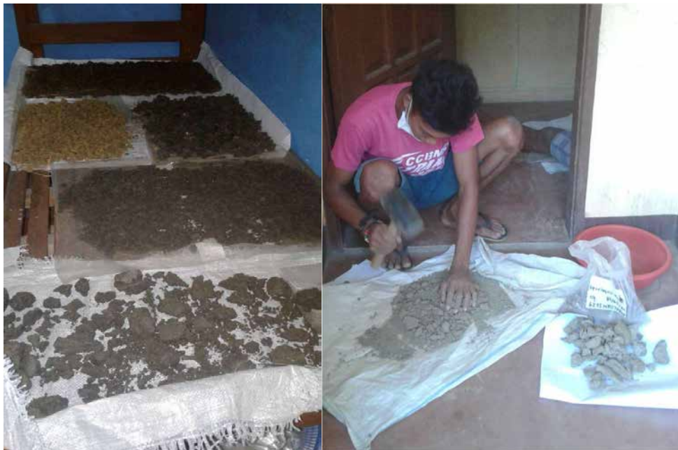
Figure 2.2 Air Drying and Pulverizing of Soil Samples
