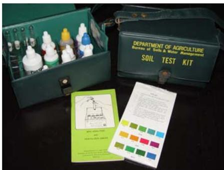
to identify quickly soil micro-nutrient problems that limit rice and other crop production. The RST also informs the user about the other new analysis required to ensure that location-specific fertilizers are recommended. The RST includes quick field
