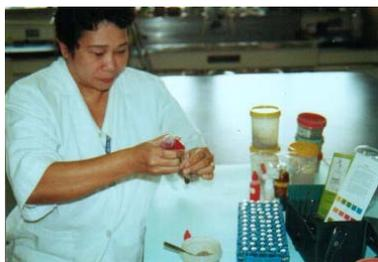
The STK is an inexpensive, quick, handy and easy to use as soil testing tool. Results are obtained within an hour. It is therefore useful to farmers and extension workers to determine on the spot what kind and amount of fertilizer to use to a grown crop in a given farm.
