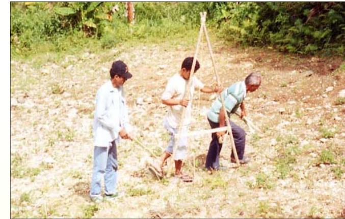
Finding contour lines using the A-Frame
