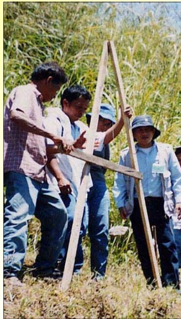
Contouring using the A-Frame, as the first step for soil conservation
